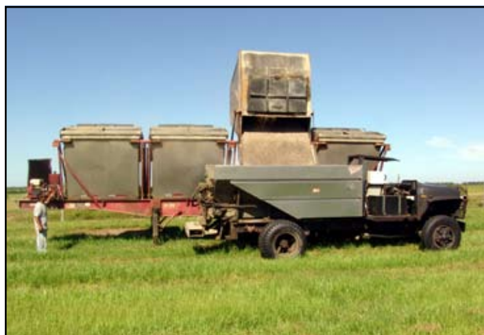
Fig. 6.1. Unloading dry solid fertilizer from a delivery trailer to a grove spreader. (Stephen Futch)
