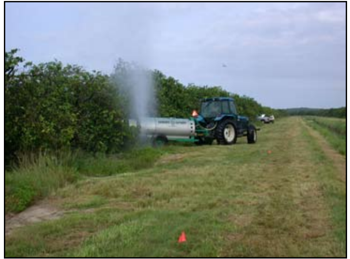
Fig. 7.5. Airblast sprayer used to apply soluble nutrients to citrus tree foliage. (P. Chris Wilson)
