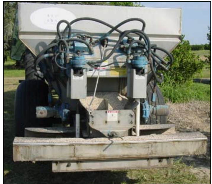
Fig. 7.1. Conventional fertilizer spreader equipped with a split chain and rear deflector plates to apply dry, solid fertilizer beneath the citrus tree canopy. (Mongi Zekri)
